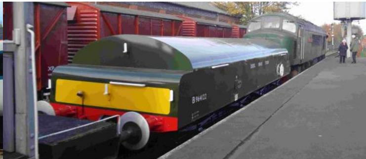
British Railways built these vehicles using redundant carriage underframes to give the new diesels extra brake force to overcome a problem the early diesels had in stopping unfitted trains.
